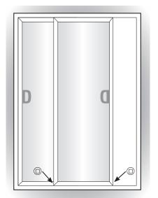
Adjust the operating panel with the screw at each end.
